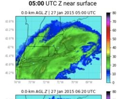
• Developing heavy snow nowcasting techniques based on polarimetric (high *K*<sub>DP</sub>) signatures aloft with over 1 hr lead time due to slow fall speed of snow
