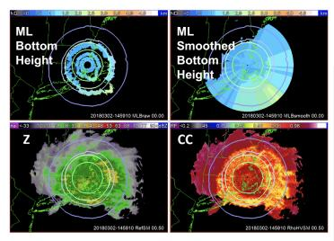
• Tested new melting layer detection algorithm with spatially variable melting layer top and bottom
