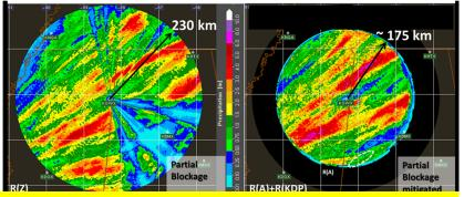
The impact of the partial beam blockage caused by nearby trees is completely eliminated in the rainfall map retrieved from A
