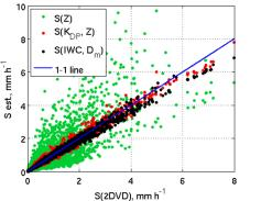
The polarimetric estimates of snow rate are much less sensitive to the variability of snow size distribution than the conventional S(Z) estimates
